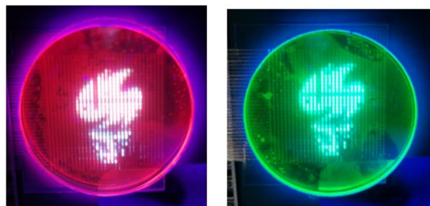
Figure 8. ( a ) The conversion effect of red quantum dot film with DBR. ( b ) The conversion effect of green quantum dot film with DBR.
